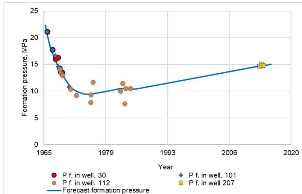
Figure 9 – Adaptation of the MBE behind the formation pressure of the known horizon wells 30, 101, 112
