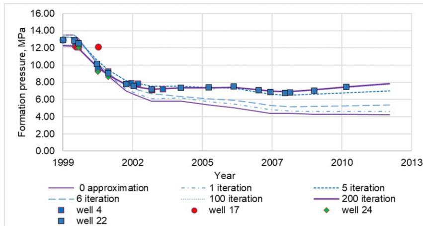
Figure 7 – Adaptation of MBE behind the formation pressure of the known horizon wells No. 4, 17, 22, 24
