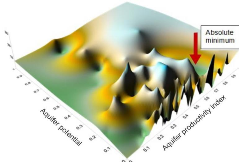
Figure 4 – The relief of the total square-law error of approximation of the reservoir pressure dynamics for the known gas reservoir of the field by the material balance equation depending on the potential and productivity index of the aquifer
