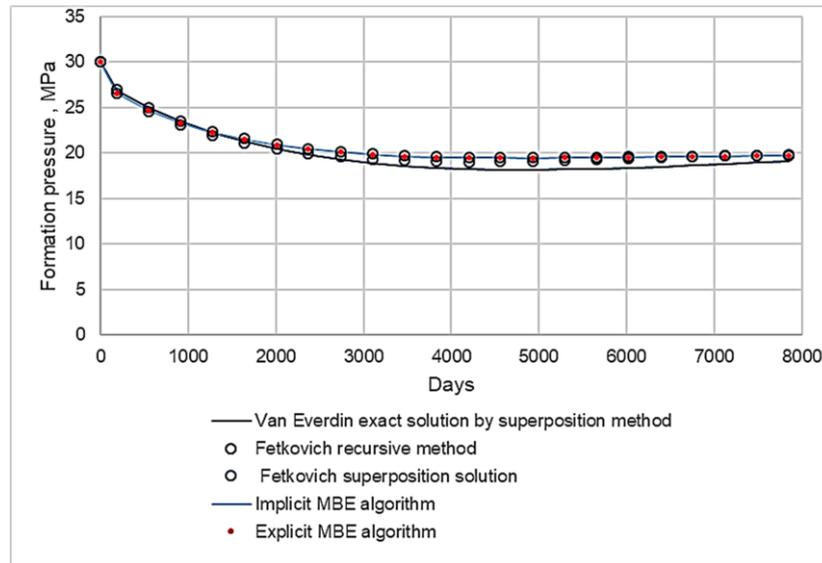
Figure 2 – Comparison of the calculated weighted average reservoir pressures for a circular reservoir R = 5
