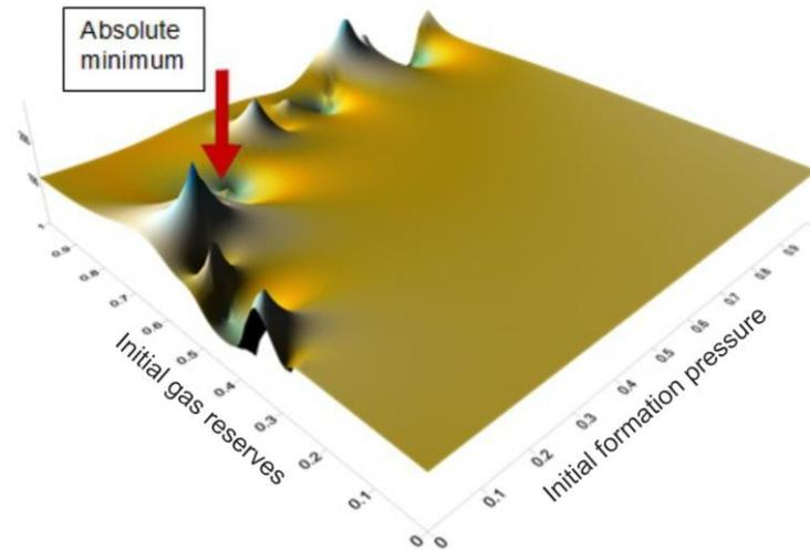
Figure 5 – Relief of the total squared error of approximating the dynamics of reservoir pressure for the known gas reservoir by the material balance equation depending on the initial gas reserves and initial pressure
