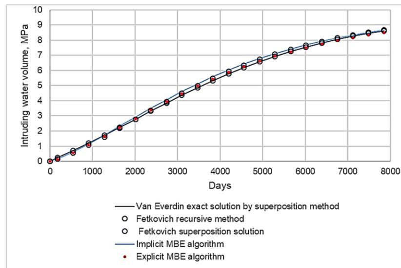
Figure 3 – Comparison of the calculated volumes of invading water for a circular formation R = 5
