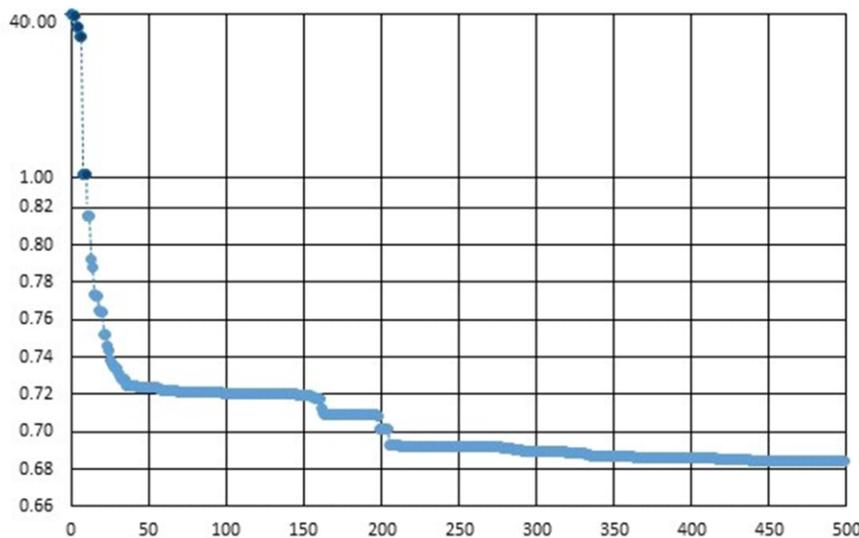
Figure 8 – Objective function dynamics depending on the number of minimizer samples
