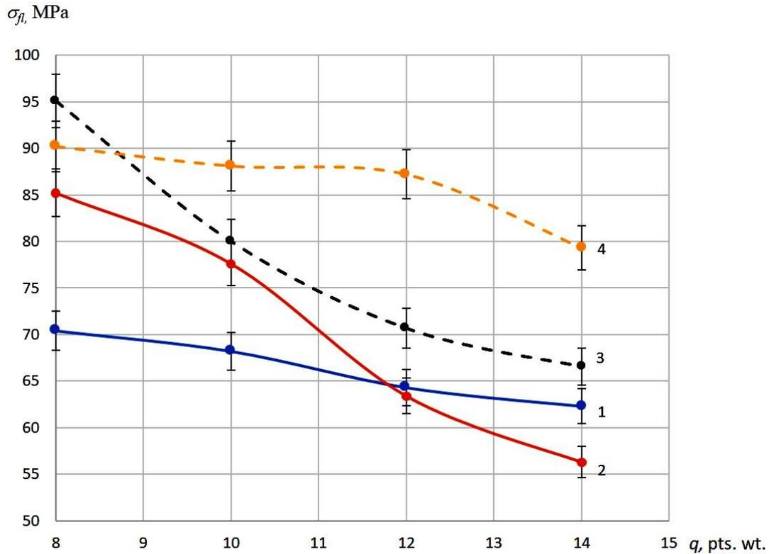
(1)  $T = 393 \pm 2 \text{ K}$  and (2)  $T = 413 \pm 2 \text{ K}$ ; fracture stresses during the flexion ( $\sigma_{fl}$ ) of the polymer matrix, hardened at a temperature: (3)  $T = 393 \pm 2 \text{ K}$  and (4)  $T = 413 \pm 2 \text{ K}$
