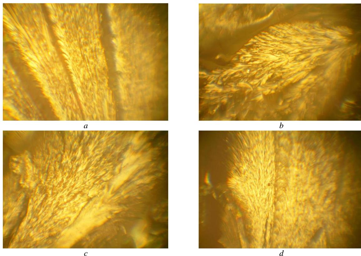
a) 8 weight parts, b) 10 weight parts, c) 12 weight parts, d) 14 weight parts
