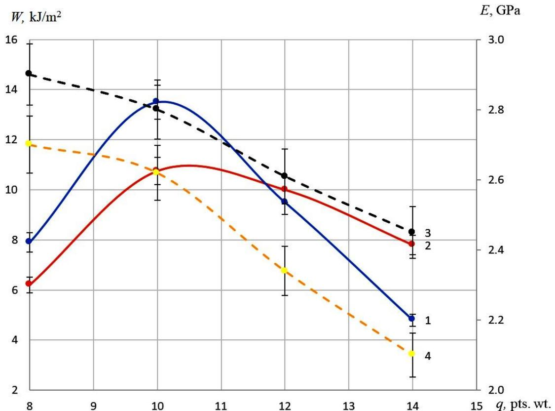
(1)  $T = 393 \pm 2 \text{ K}$  and (2)  $T = 413 \pm 2 \text{ K}$  – the modulus of elasticity during the flexion ( $E$ ) of the polymer matrix, hardened at a temperature: (3)  $T = 393 \pm 2 \text{ K}$  and (4)  $T = 413 \pm 2 \text{ K}$
