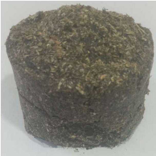
Figure 1 – Pressed briquettes based on the secondary products of plant processing
