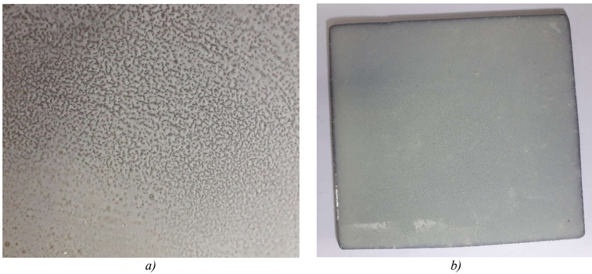
Figure 6 – General view of a layer of epoxy composite coating modified with polyvinyl chloride with a solvent content
