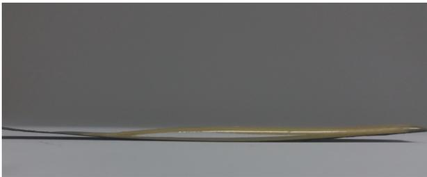
Figure 3 – Defects of the coating caused by high residual stresses
